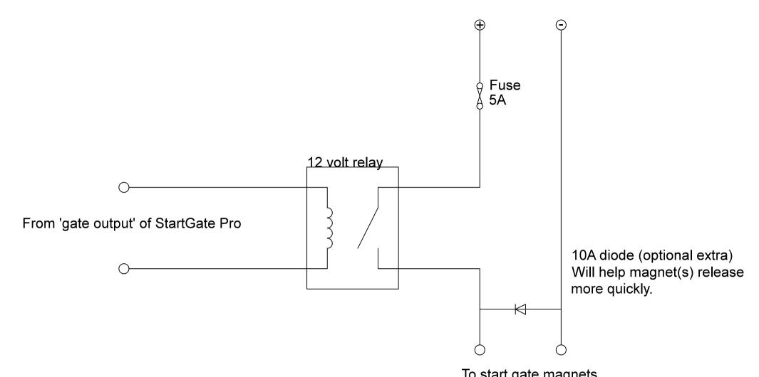
The 5A fuse is essential to protect the wiring from a short circuit. Car batteries can deliver hundreds of amps. The diode is not essential, but can be used to help the magnets release more quickly, by giving the back EMF from the magnets a path to flow.
